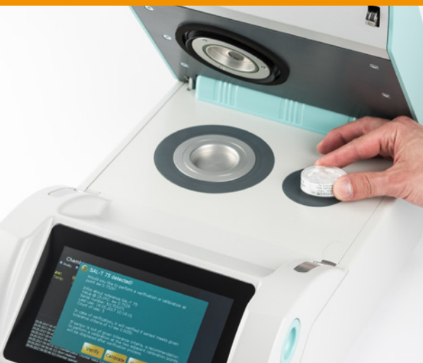
Left: Simple traceable calibration with RFID re-usable salt capsules. By swiping the salt over the chip reader, the calibration is automatically started.
